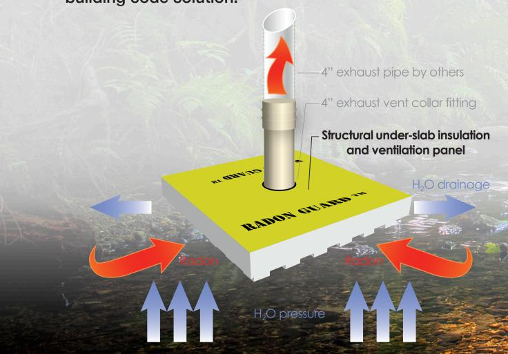
Radon Guard<sup>™</sup> combined with the polyethylene membrane Radon Block<sup>™</sup> provides a level of protection far superior to existing standard building materials.
